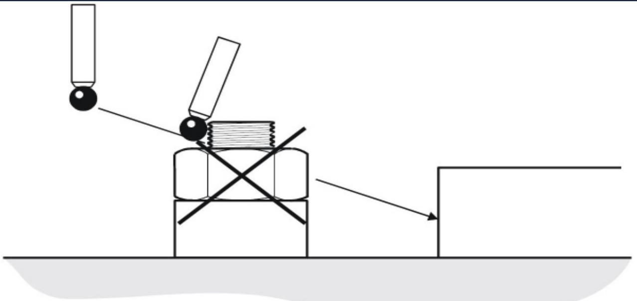
Using intelligent "protected moves" built into the Renishaw macros, we position the probe in any location around the tombstone and move at a speed that avoids damage to the probe even if the part is drastically out of position. Should the probe collide with anything while running Renishaw program o8810, the probe stops before damage occurs.
