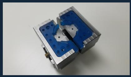
CSP prides itself on being at the forefront of technology in modern manufacturing. We have used 3D printers shop-wide to automate QC inspections and provide set-up jigs and fixtures for our Fanuc Robotic arms. 3D printed workholdings pose new challenges while opening new opportunities to engage with lower volume customers.
